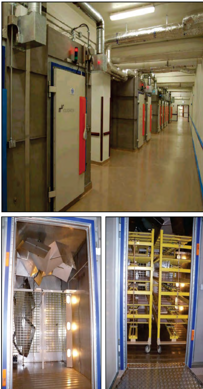
FIGURE 3 Exterior View of Chambers, Empty Chamber Showing the Vertical and Horizontal Stirrers, and Chamber with Cage Racks in Place
